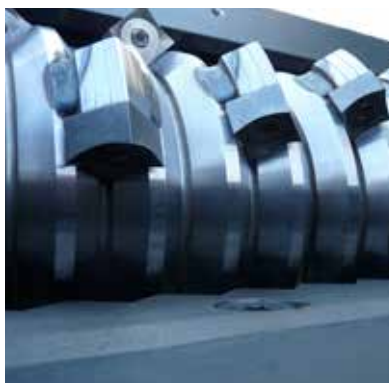
Rotor with double row of blades
