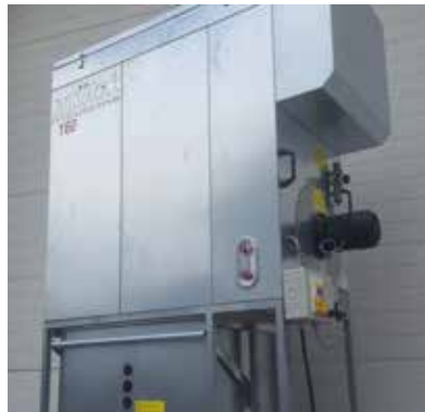
Extraction unit MMJet 160 with mobile container
