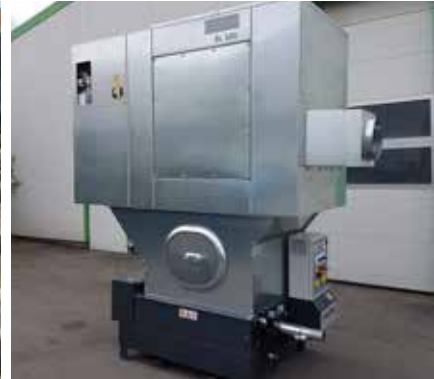
Extraction unit MMJet 300 with briquetting press
