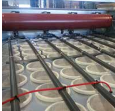
Option: Automatic, compressed air cleaning system
