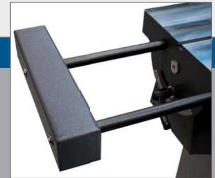
⊙ : LEFT AND RIGHT SLIDE SUPPORT 400 MM
