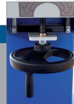
S: MECHANICAL ADJUSTEMENT OF SPINDLE HEIGHT
