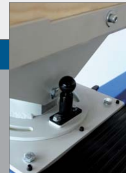
S : FIXING OF SPINDLE IN WORKING ANGLE
