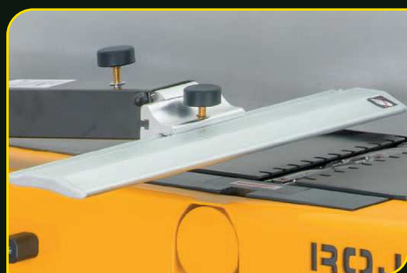
CPS cover of cutterblock CPS Messerwelleschutz
