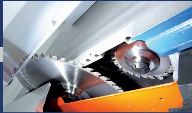
Vorritzaggregat AUTO-EPS in Parkposition • Scoring saw aggregate AUTO-EPS in parking position • Grupo incisor AUTO-EPS en la posición de aparcamiento
